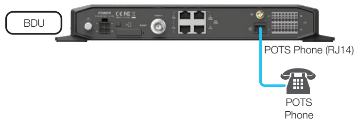
Figure 31: BDU to POTS Phone (RJ14) Cable Connection
