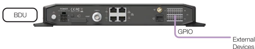
Figure 33: BDU to External Devices Connection
