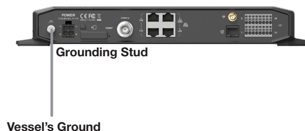
Figure 31: Grounding Stud Connection
