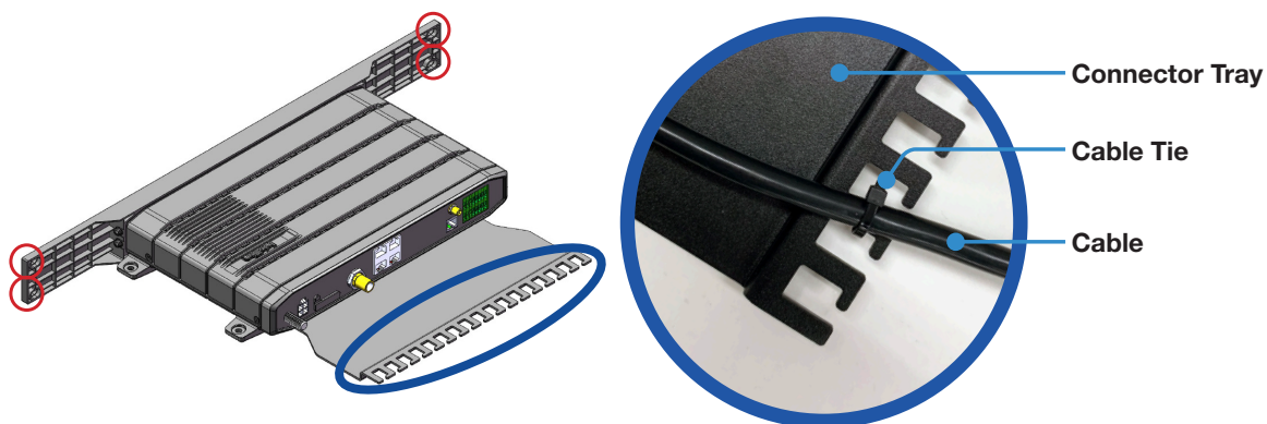
Figure 22: Mount BDU Assembly into 19" Rack
