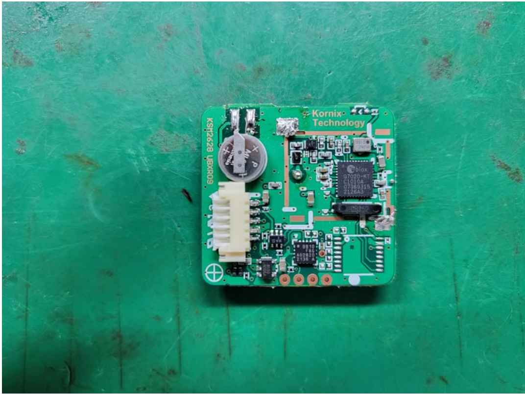
GPS Mainboard front (shielding removed)
