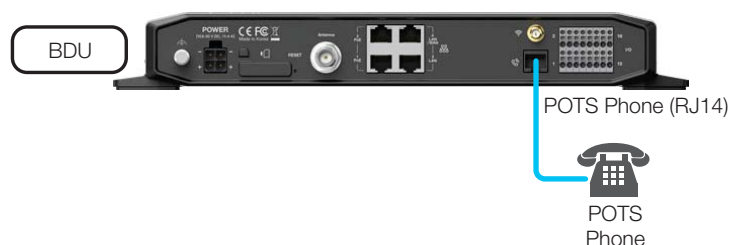
Figure 39: BDU to POTS Phone (RJ14) Cable Connection
