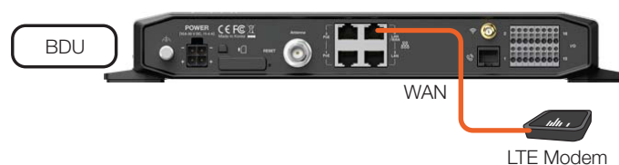
Figure 38: BDU to Device Cable Connection using WAN Port
