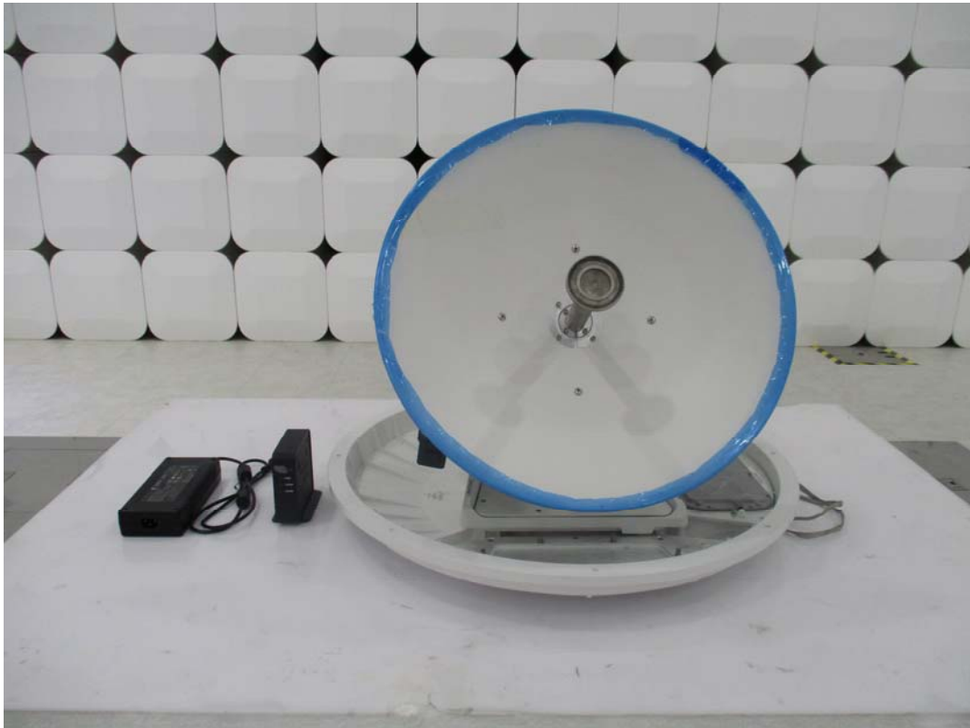
PS-OW50SP(Antenna Unit, CNX)
