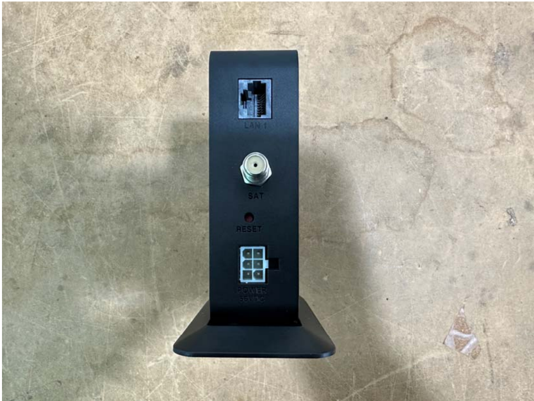
Customer Network Exchange I/O port
