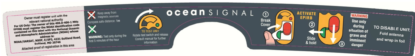
Figure 1: E101V EPIRB Front Label with Operating instructions
