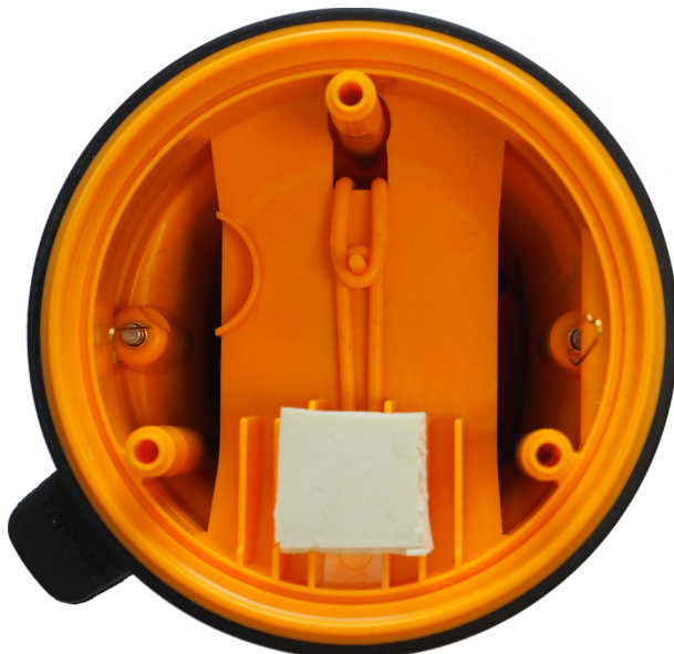
Figure 2: rescueME EPIRB1 – Top view, PCB removed, showing battery carrier in situ.
