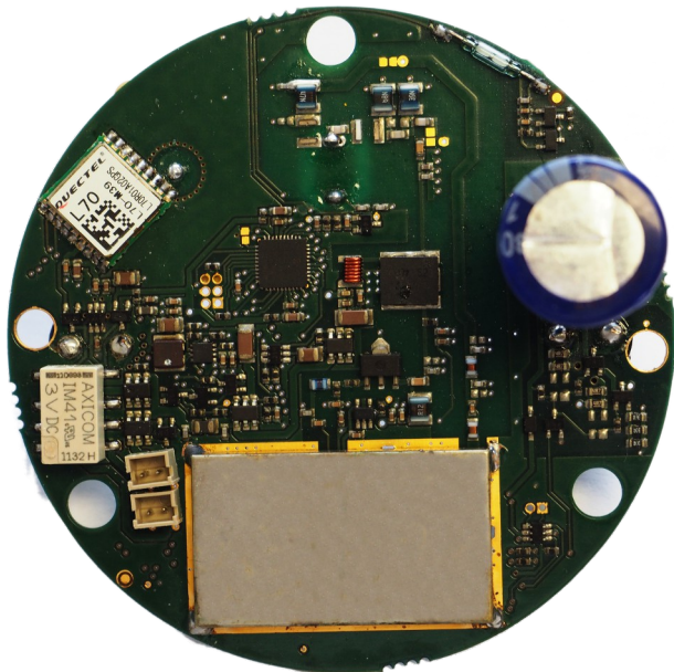
Figure 4: rescueME EPIRB PCB – Rear side
