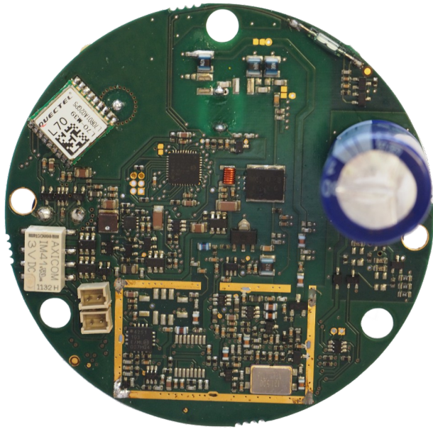
Figure 5: rescueME EPIRB PCB – Rear side with screening can removed.
