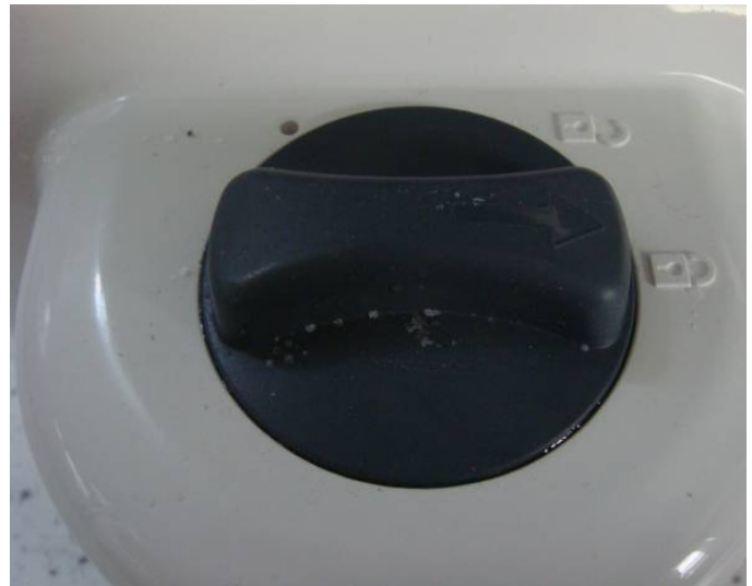
Figure 6.8 – View exterior inspection of EUT (EPIRB) upon completion the salt fog test
