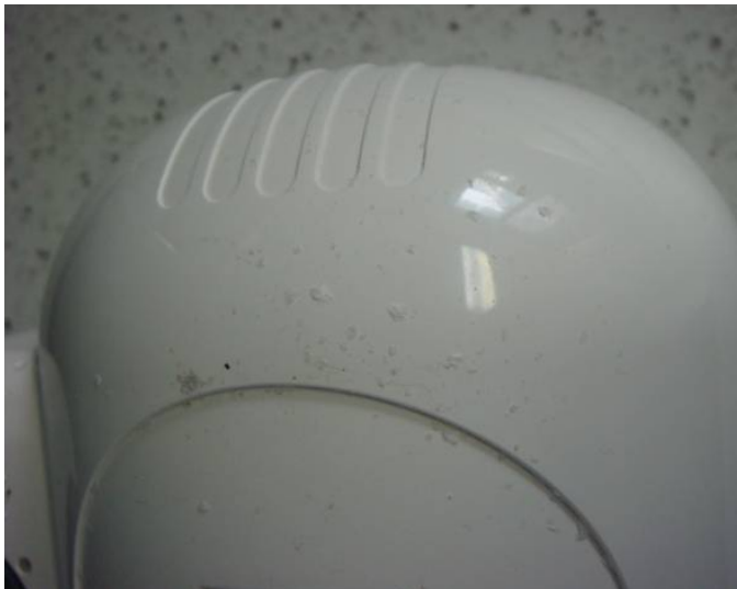
Figure 6.8 – View exterior inspection of EUT (EPIRB) upon completion the salt fog test
