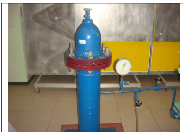
Figure 9.1 – View of immersion test site (Manometer of immersion test site indicates 1 bar)
