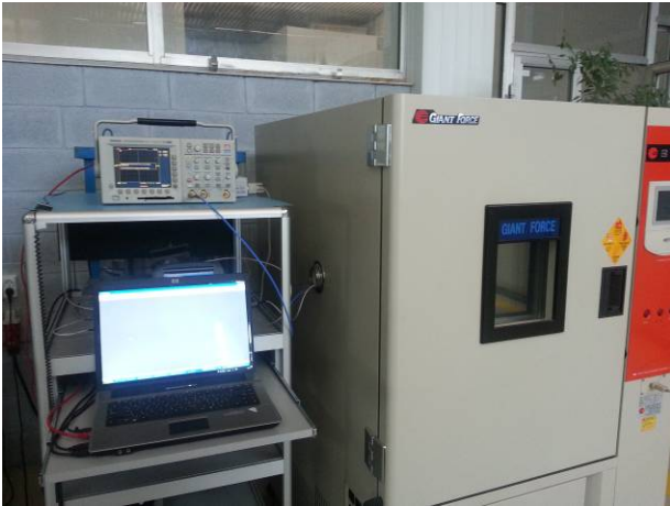
Figure 13.2 – Site for Carrier Frequency Test and Modulation Characteristic Measurement at the minimum, ambient and maximum operating temperatures
