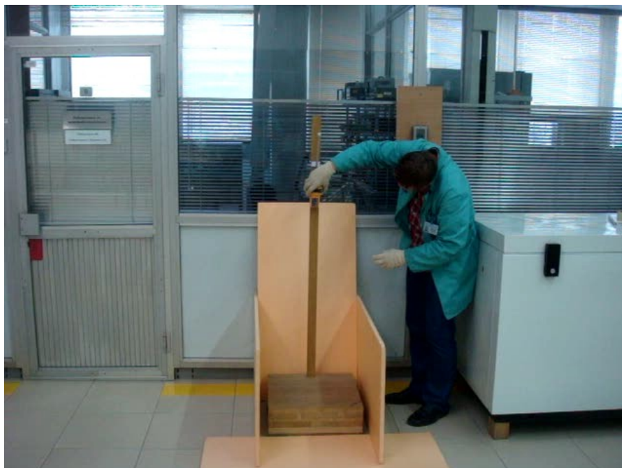
Figure 7.1 - Total view of test site of the drop from a height of 1 m above the test surface
