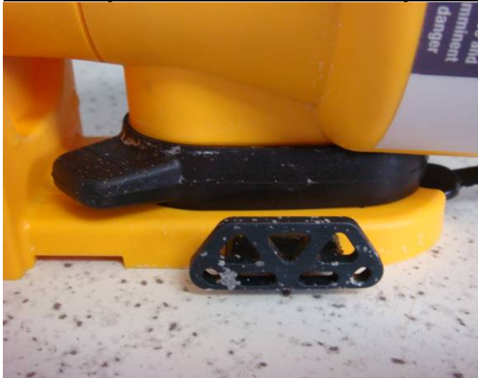
Figure 6.7 - View exterior inspection of EUT (EPIRB) upon completion of the salt fog test
