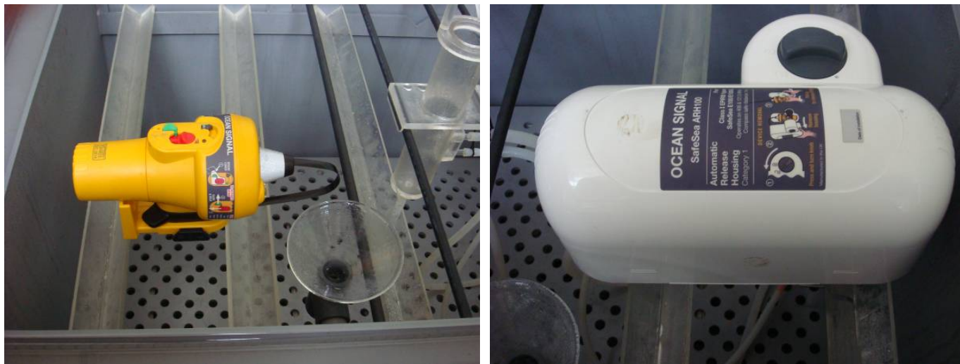
Figure 6.1 - Views of the EUT (EPIRB) before the salt fog test
