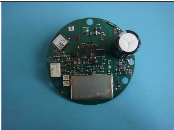
Figure 9.2 – The PCB after leakage and immersion tests. There is no water ingress.
