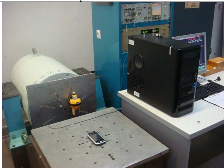
Figure 5.7 - General view of the horizontal X vibration test (EPIRB1 with Manual Bracket)
