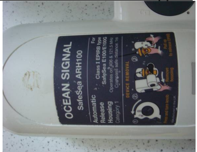
Figure 6.7 - View exterior inspection of EUT (EPIRB) upon completion of the salt fog test
