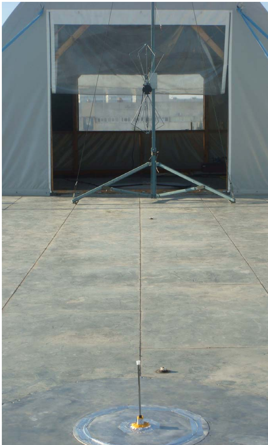
Figure 1. The photograph of the site (OATS No.33) for measurements of 121.5 MHz Peak Effective Radiated Power
