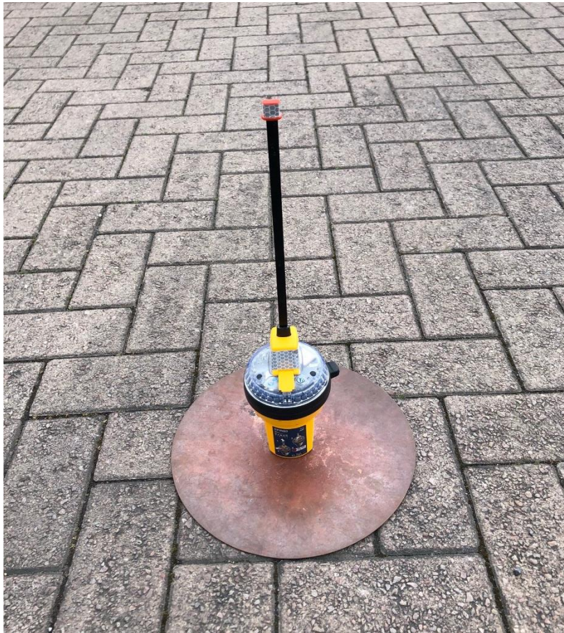
Position Acquisition Time and Position Accuracy Test – Configuration 7 – A.3.8.2.1 EPIRB2 Pro
