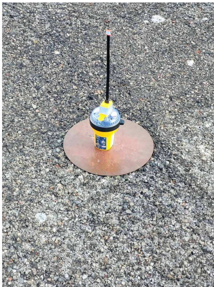
Satellite Qualitative Test – Configuration 7 EPIRB2 Pro
