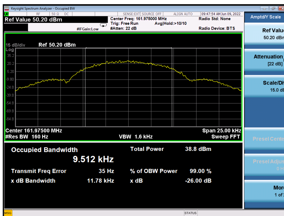
Figure 1 – 161.975 MHz Occupied Bandwidth
