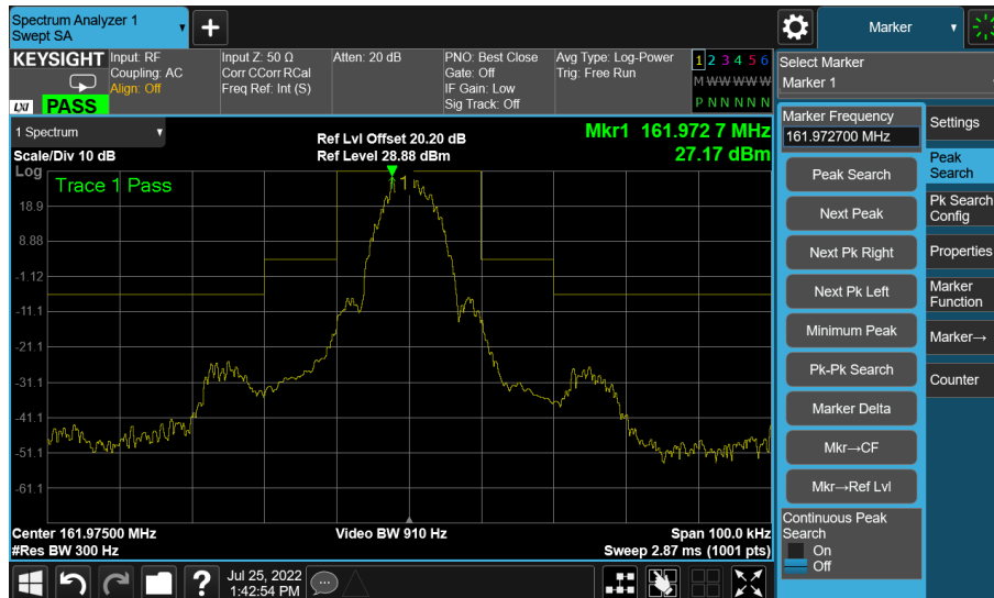
Figure 3 – 161.975 MHz - Transmitter Spectrum Mask
