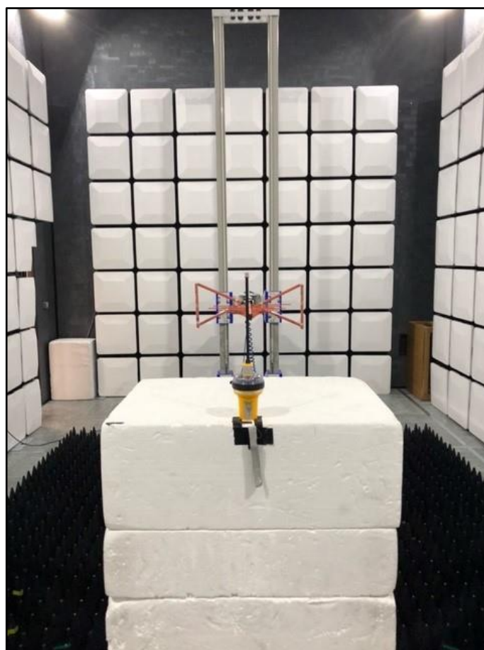
Figure 41 – 1 GHz to 2 GHz, Y Orientation
