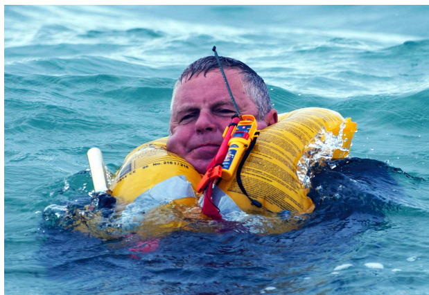
Figure 6 MOB1 showing antenna deployed and typical operational situation
