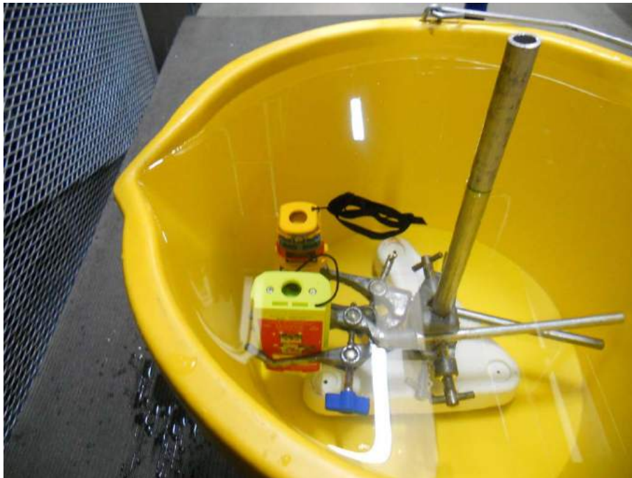
Test Setup (1-hour immersion)
