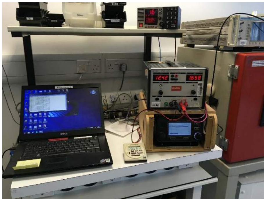
Battery Capacity Test Monitoring Equipment
