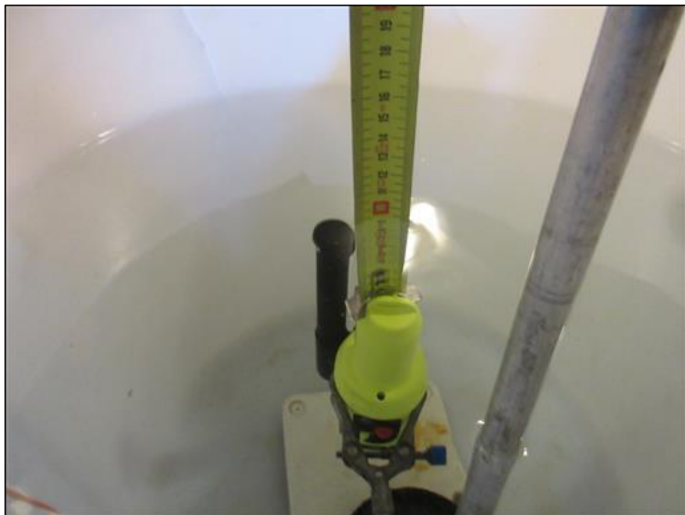
Figure 31 - Test Setup – EUT submerged (depth check)
