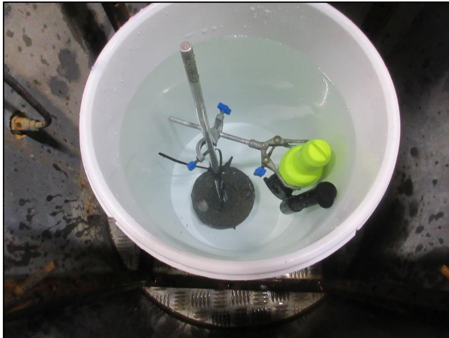
Figure 43 - Test Setup – EUT submerged in pressure chamber
