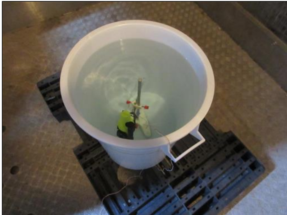
Figure 24 - Test Setup – EUT in Chamber (EUT immersed in water at +25°C)
