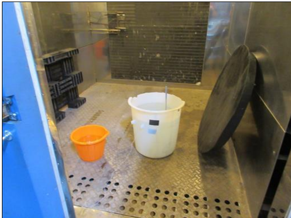
Figure 32 - Test Setup (EUT immersed in water at +25°C)
