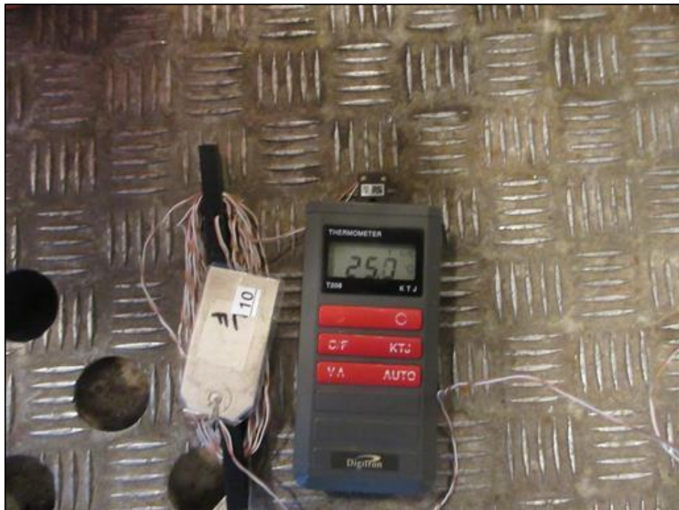
Figure 30 - Test Setup - Water temperature check prior to submersion - 25.7c
