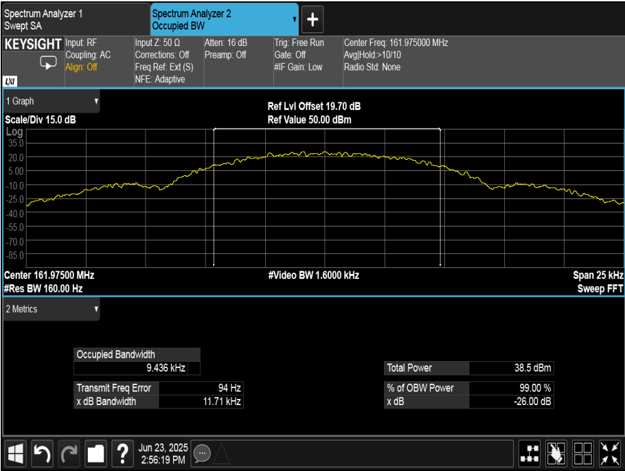
Figure 3 - 161.975 MHz Occupied Bandwidth
