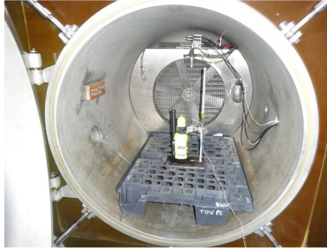
Test Setup – EUT in Chamber (Conditioning at +70°C)
