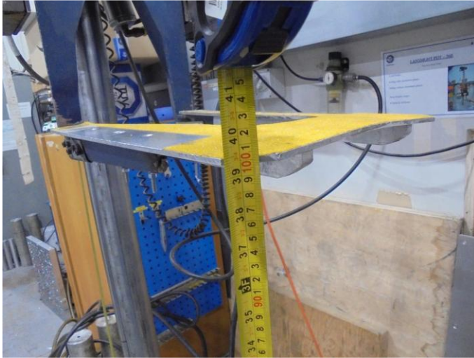
Drop Height 1000 mm Measurement
