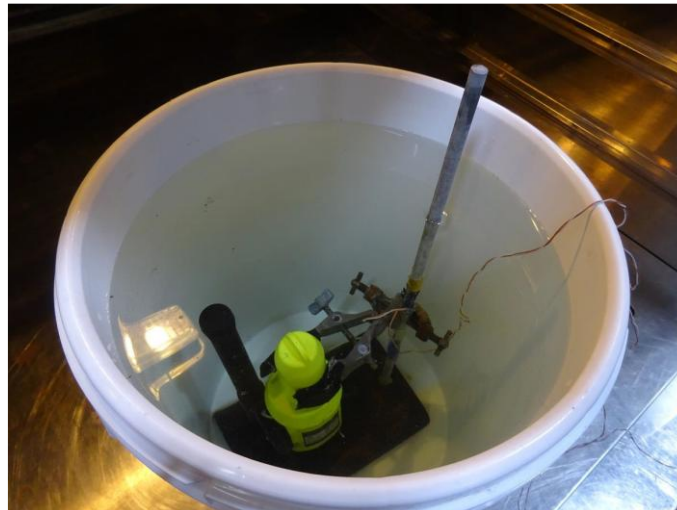
Test Setup – EUT in Chamber (EUT immersed in water at +25°C)
