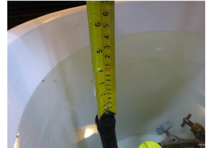
Test Setup – Water Depth to EUT
