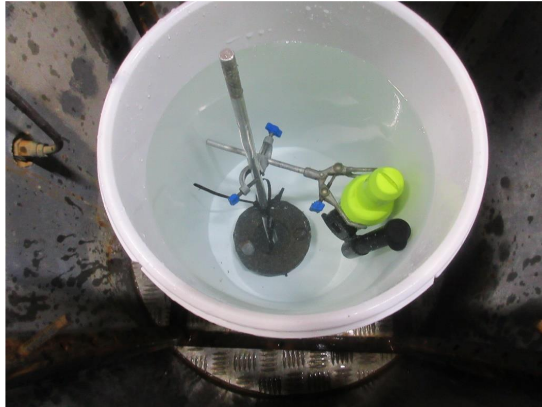
Test Setup – EUT submerged in pressure chamber
