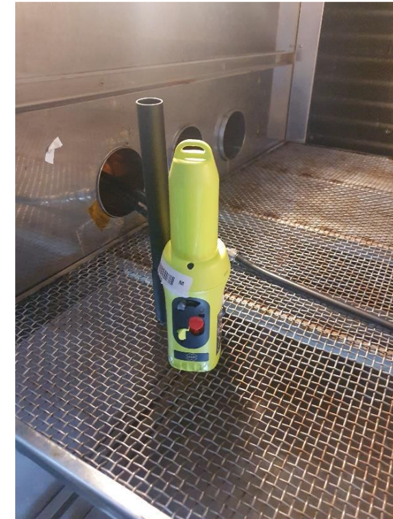
Damp & Low Heat Test Setup EUT in Chamber
