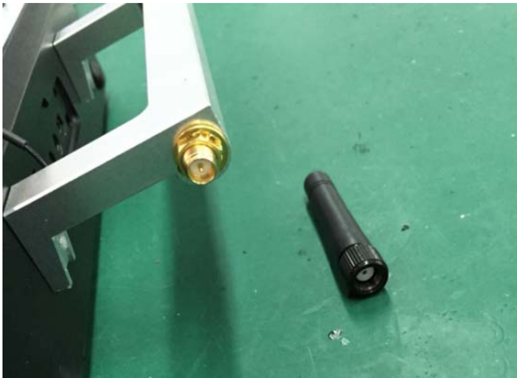
SMA Port – Front View
