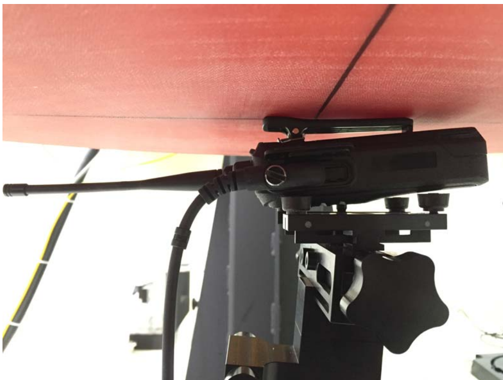
Body-worn, the front of the EUT towards ground with A1, B1,BC1,S1 and D1 (The distance was 0mm)
