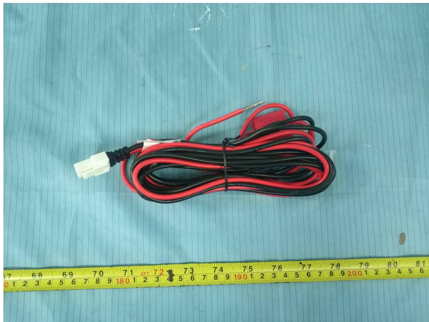
EUT – DC Cable View
