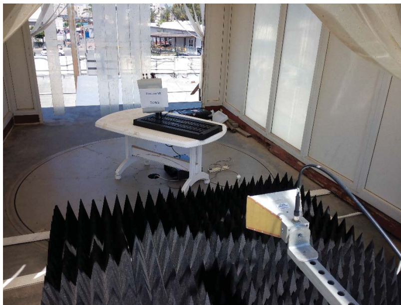
Figure 5. Spurious Radiated Emission Test – 1-7GHz
