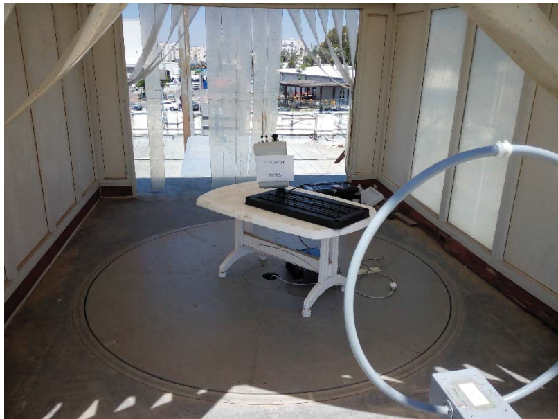
Figure 3. Spurious Radiated Emission Test – 9kHz-30MHz
