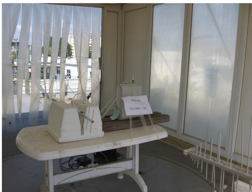
Figure 4. Radiated Emission Test in the band 602MHz-620MHz
