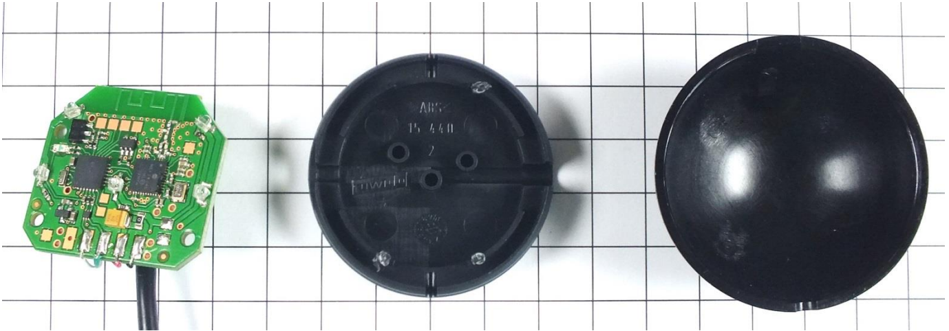
Interior view of housind and PCB
