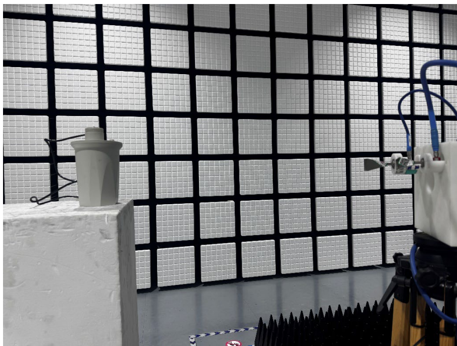
Description: Radiated Emission Test Setup (Above 18GHz)
