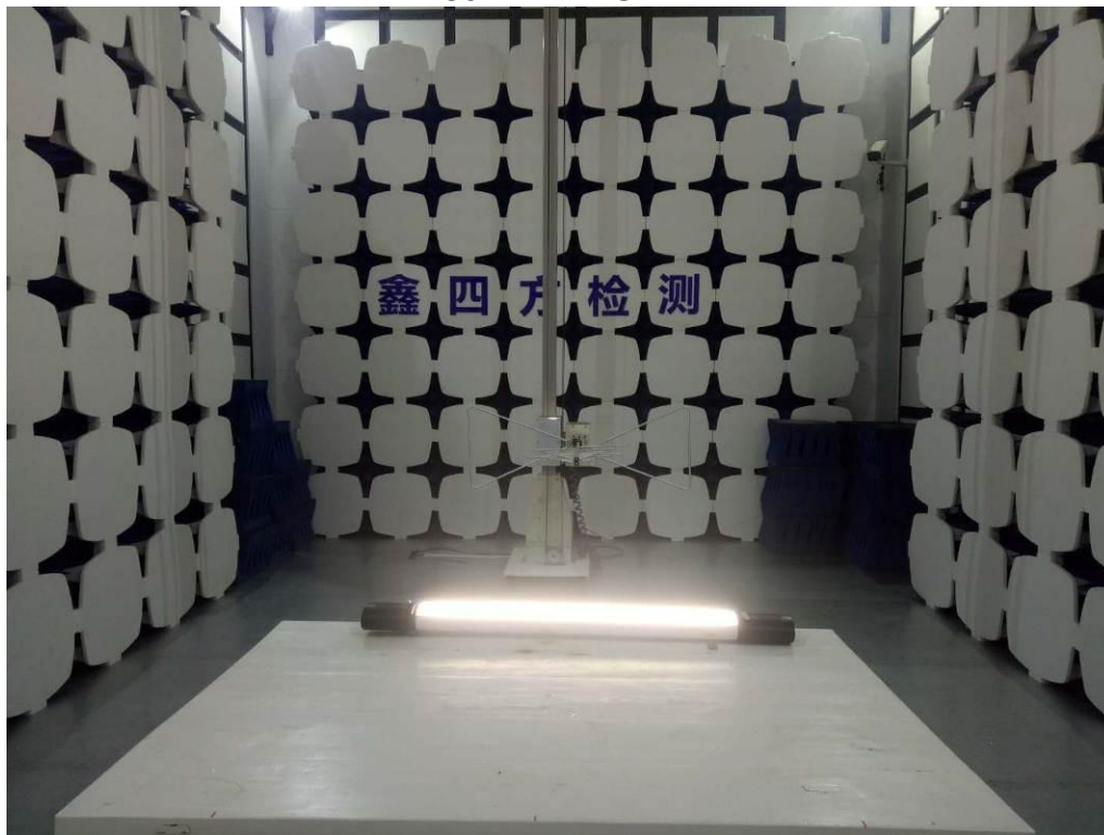
Photos of radiated emission test 30MHz – 1GHz
