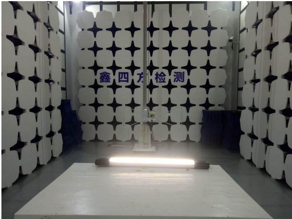
Radiated emission test 30MHz – 1GHz
