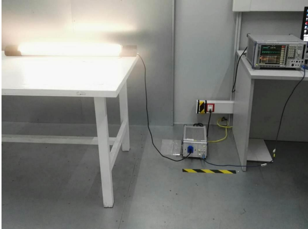
Radiated emission test 30MHz – 1GHz
