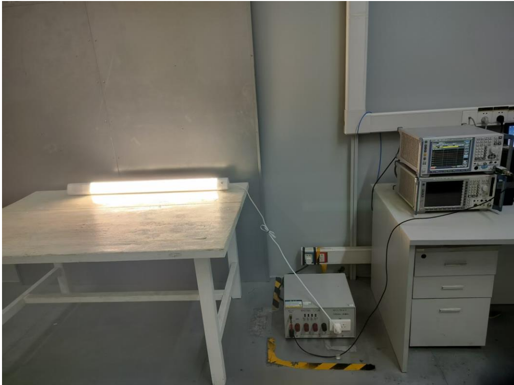
Photos of power line conducted emission test
