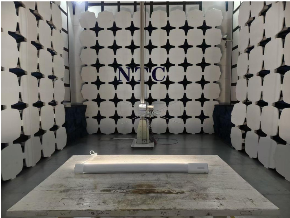
Photos of radiated emission test 30MHz – 1GHz
