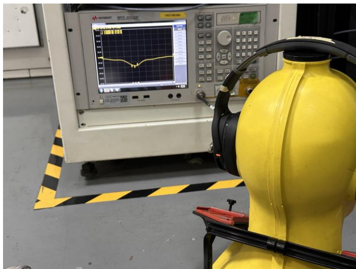
Free Space Impedance Setup
