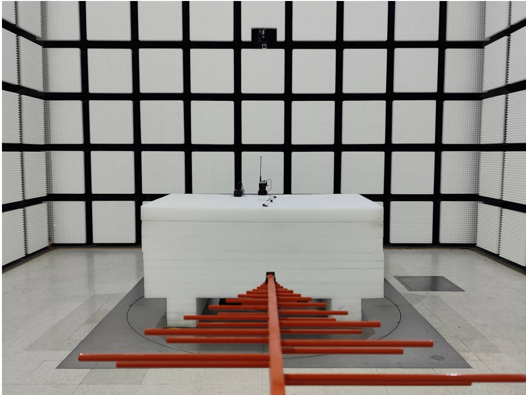
Radiated Emission Below 1GHz rear View M2
