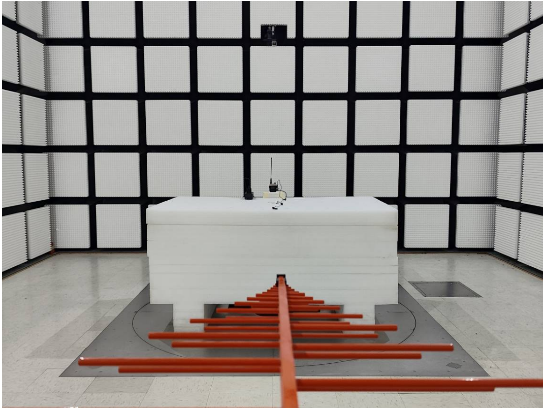
Radiated Emission Below 1GHz rear View M1
