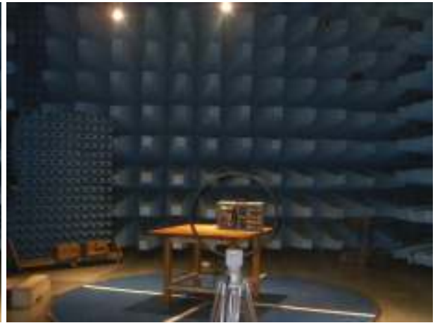
Loop antenna (9kHz ÷ 30 MHz) measurement distance: 3 m
