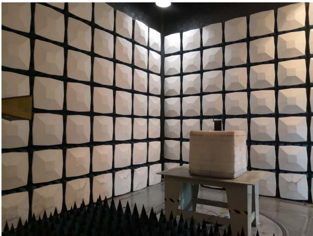
Radiated Emission Above 1GHz View
