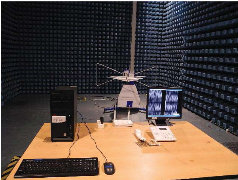
Photo 2 Radiated Disturbance Test
