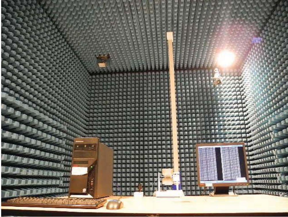
Photo 3 Radiated Disturbance Test
