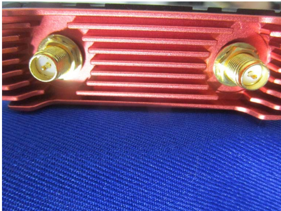
EUT -7059 Transmitter Antenna Port View
