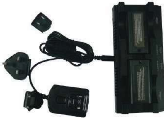
Fig. 3.6 - S9III PLUS charger and adaptor
