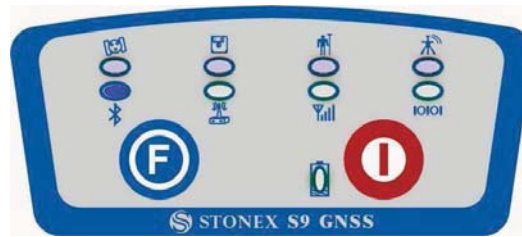
Fig 2.12 - S9III PLUS Bluetooth led
