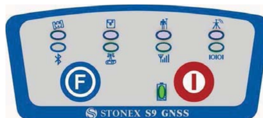
Fig. 2.16 - S9III PLUS power led
