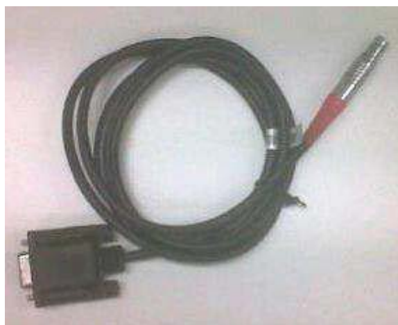
Fig. 5.24 – Cable for serial port forwarding
