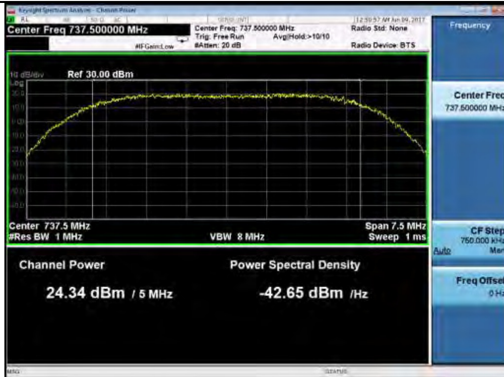
5M 64QAM Mid
