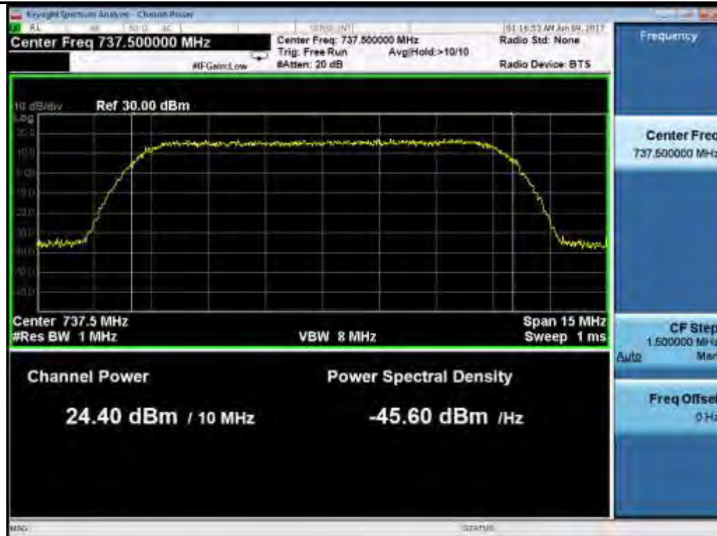
10M 64QAM Mid
