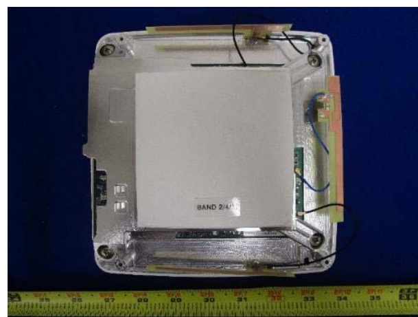
Internal Antenna View 1
