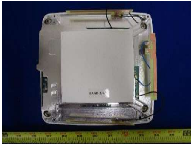
Internal Antenna View 1
