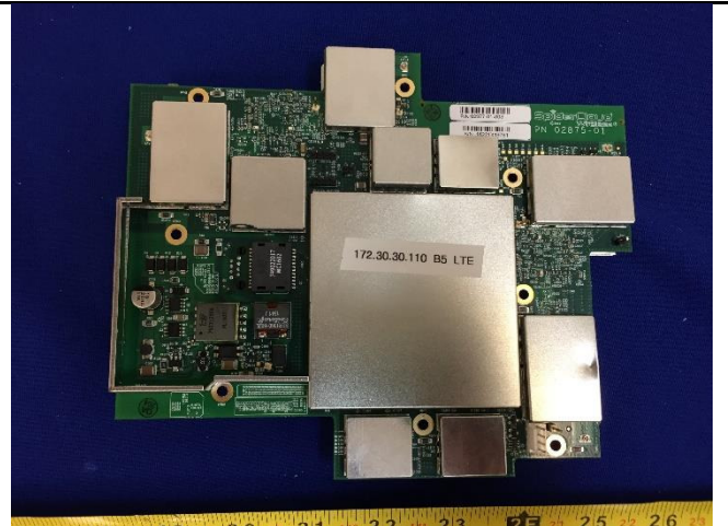
Main PCB with shielding - Top View
