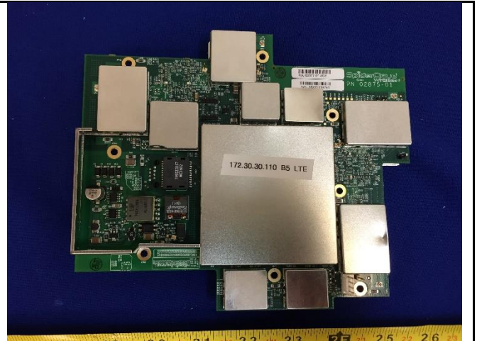
Main PCB with shielding - Top View
