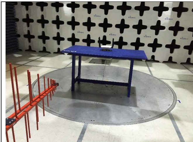
Radiated Emissions (<1GHz) – Front View
