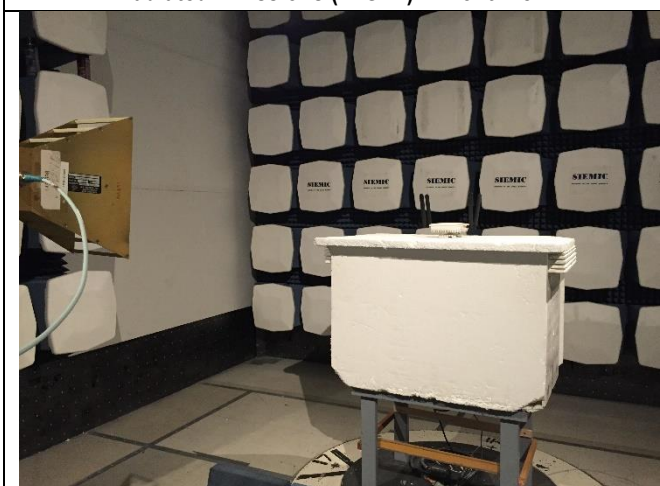
Radiated Emissions (>1GHz) – Front View
