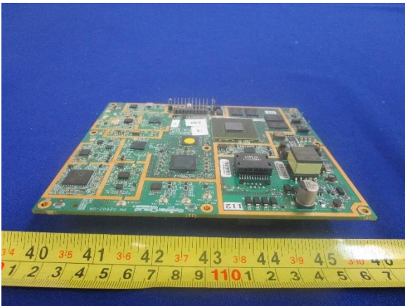
Picture 5: Main Board- Rear View
