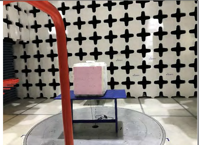
Radiated Emissions (<1GHz) – Rear View
