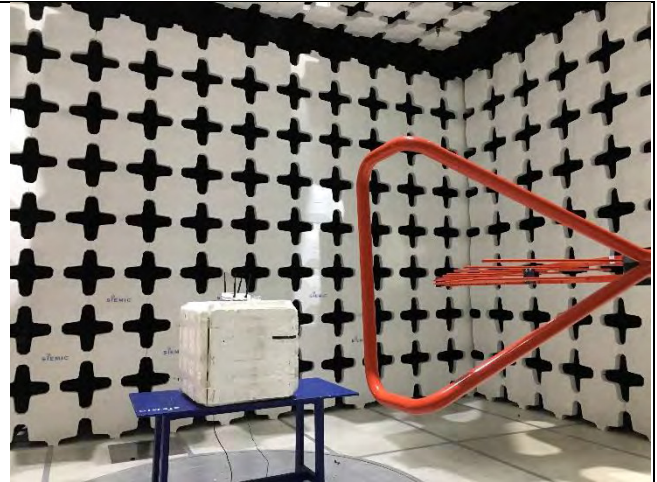
Radiated Emissions (<1GHz) – Rear View
