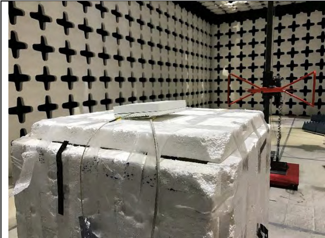
Radiated Emissions (<1GHz) – Front View
