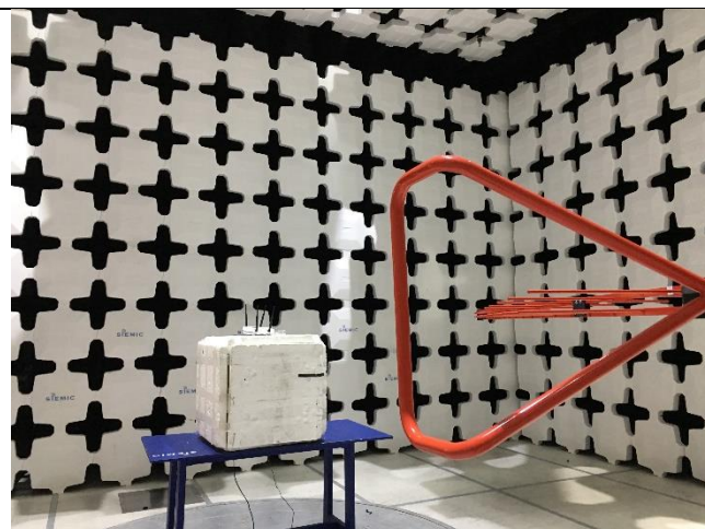
Radiated Emissions (<1GHz) – Rear View
