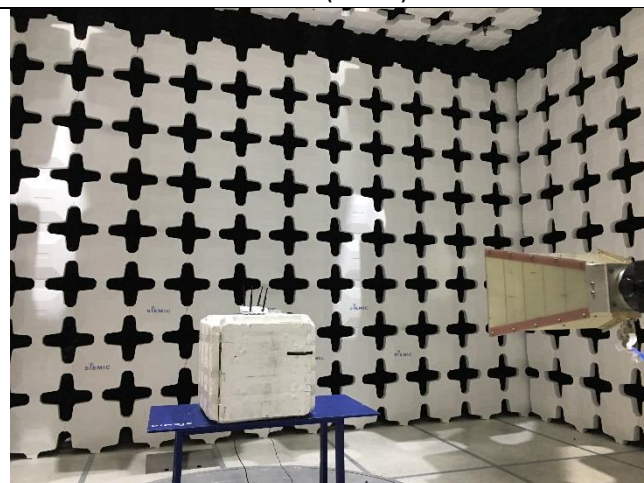
Radiated Emissions (>1GHz) – Rear View
