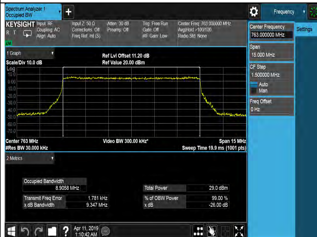
10M 64QAM Mid
