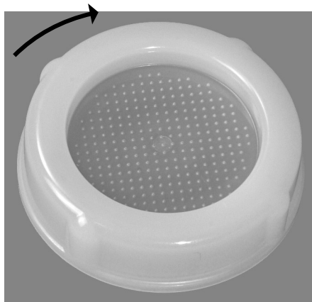
Figure 3-10: Screwing on the sampling grid
