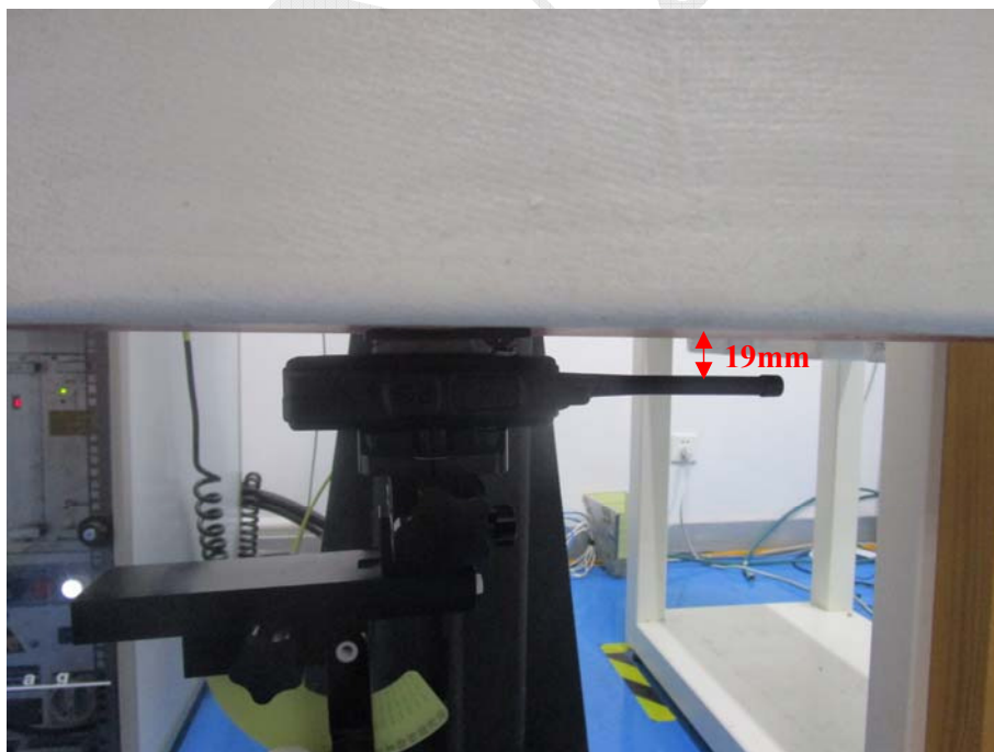
Body Worn Back With Setup Photo_ DR7800-1_148-174 MHz (0mm)
