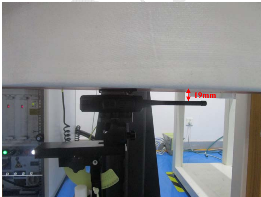
Body Worn Back With Setup Photo_ DR7800-1_136-150 MHz (0mm)
