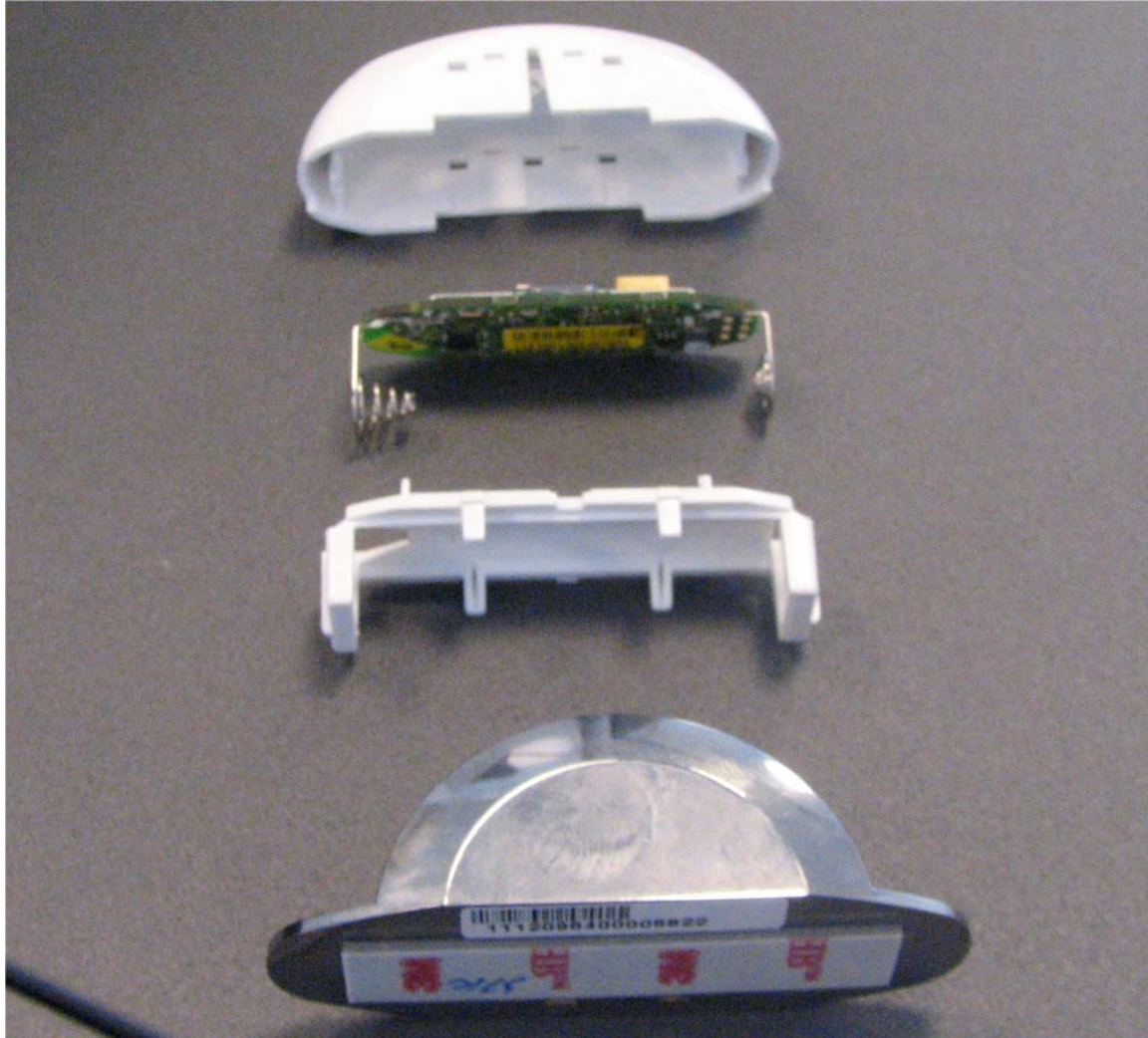
Photograph No.1 M800MGL magnet sensor (detector) internal view
