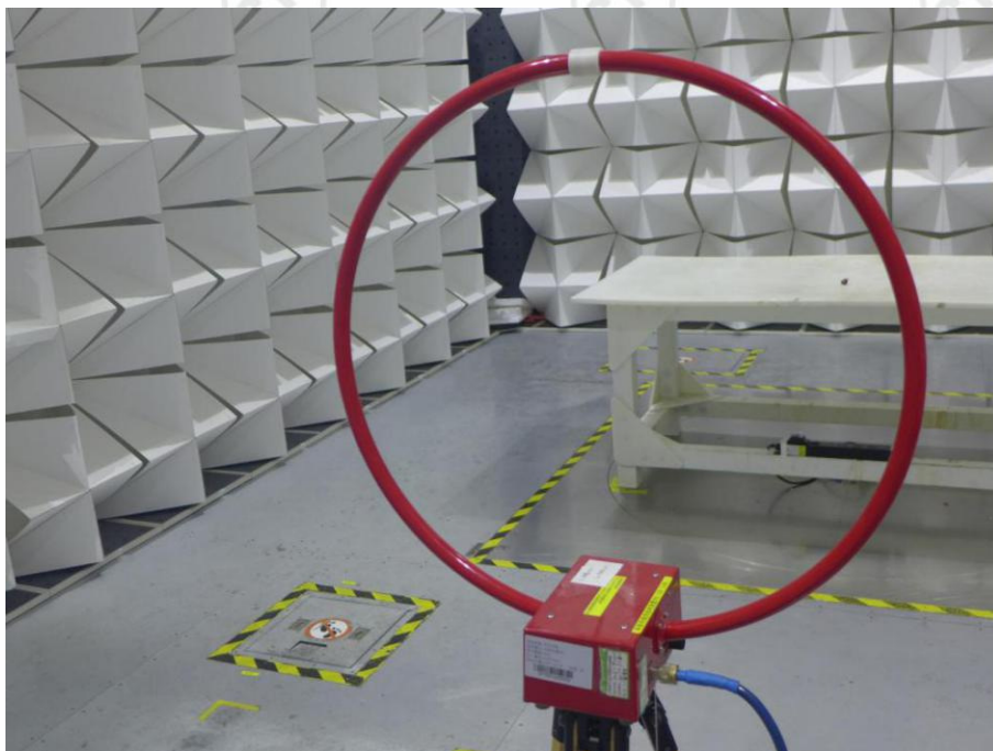
Radiated spurious emission Test Setup-1(Below 30MHz)
