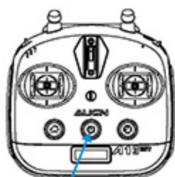
Power on A13 開啓遙控器電源
