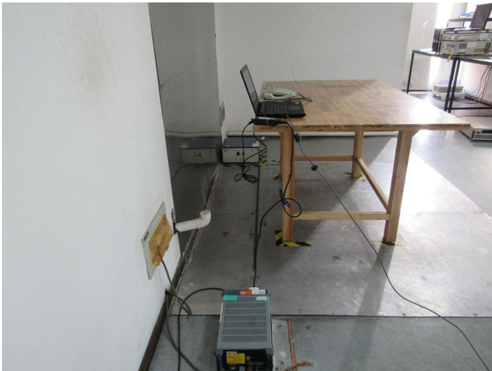
Conducted Emissions Test Setup Side View (Notebook)
