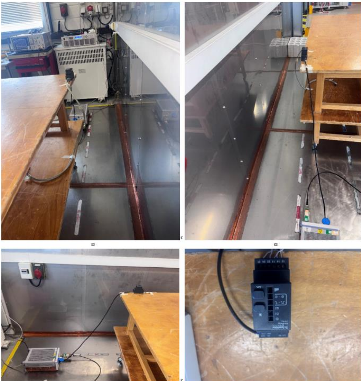
Photo of AC Power Line Conducted Emissions (direct)
