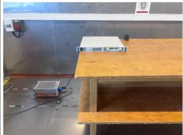
Photo of AC Power Line Conducted Emissions (120 VAC / 24 VDC via PSU)
